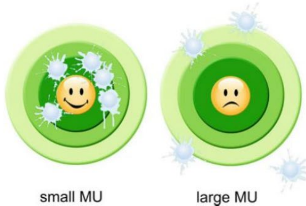
Fig. 17 Results of repeated measurements of the same sample can give very distributed values around target value, representing large MU, whereas results concentrated near the target value represent small MU
